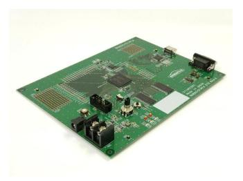
The RH850/D1M1A ETS board is an evaluation board equipped with the microcomputer RH850/D1M1A (Renesas, R7F701461).
