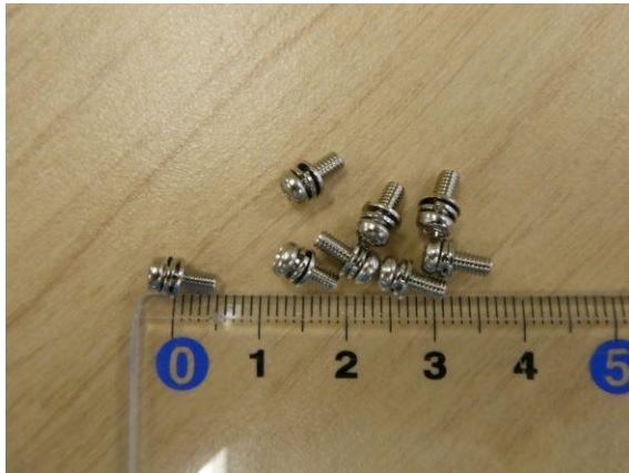
Picture 2-10 M2.6 pan head screw: 9 B-2606-S1 (1 spare)
