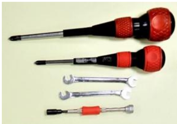
Picture 2-13 phillips screwdriver(L[M3], M[M2.6]), wrench(5mm、6mm), nut driver(5mm)
