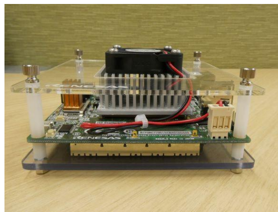
Picture 3-3 remove spacers, screws, and the acrylic plates from R-Car Starter Kit
