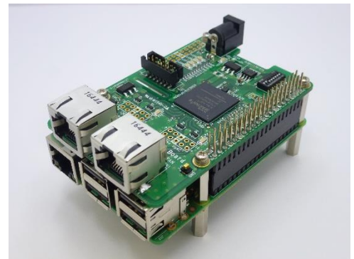
Stack SpaceWire Pi on Raspberry Pi
